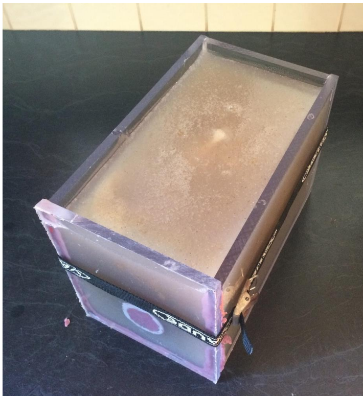
Figure 5 the filled, cooling phantom using natural Metamucil.
