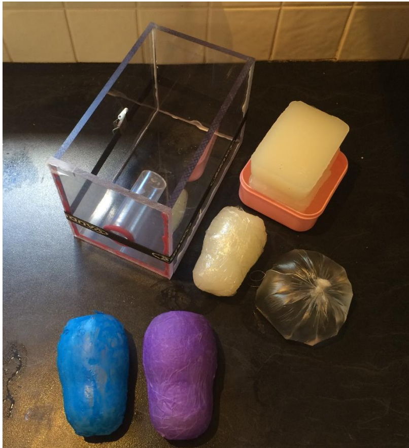
Figure 3 case, plastic bag bladder and three uterine models - blue Plasti-dip, purple paper mache and white gladwrap. Several rectangular agar blocks were used for positioning of the uterus in relation to the vaginal canal positive
