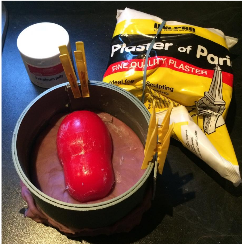
Figure 1 Making the plaster half mould
